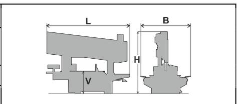
Note: The saw is divided for transport into two sections: saw and conveyor: B1 (saw) = 17 mm, B2 (conveyor) = 3000mm
